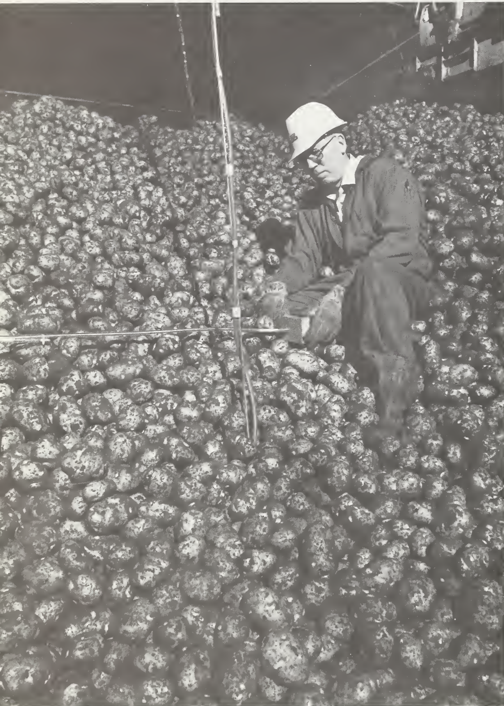
Agricultural engineer Lewis Schaper inspects vertical and horizontal air sampling tubes during bin-filling operation. (1086X1152-27)
